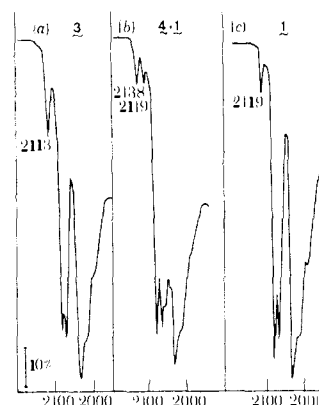
Figure 4. Key: (a) IR spectrum ( \nu_{\text{CO}} region) of 3 ; (b) after treatment with \text{H}_2 [25 °C ( 3.2 \times 10^4 Pa)]; (c) after evacuation of (b) [25 °C ( 10^{-2} Pa)].
